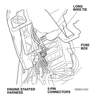
54. Slide the other clip on the engine starter harness onto the vehicle connector. Note the direction and the orientation of the clip.
