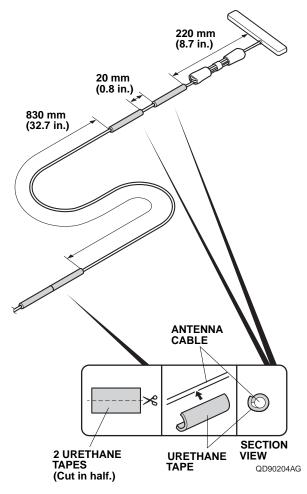
30. Wrap three halves of urethane tape around the antenna cable at the measurements shown.
