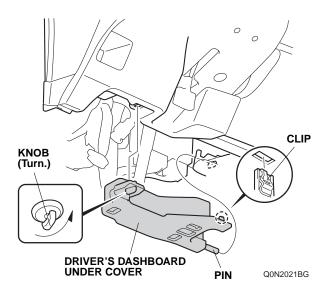
15. Remove the driver's dashboard lower cover and unplug the vehicle connectors.
