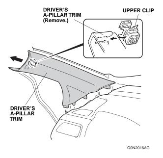
10. Remove the remaining upper clip from the driver's A-pillar.
