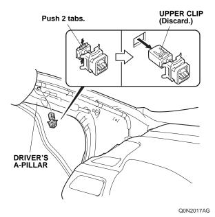
11. Temporarily reinstall the driver's A-pillar trim, and check the overlap between the headliner and the driver's A-pillar trim according to the service manual. Remove the driver's A-pillar trim. Install the new clip (supplied) to the driver's A-pillar trim.
