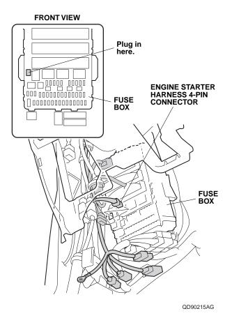
56. Unplug the fog light 4-pin connector from the fuse box, and plug it into the engine starter harness 4-pin connector.
