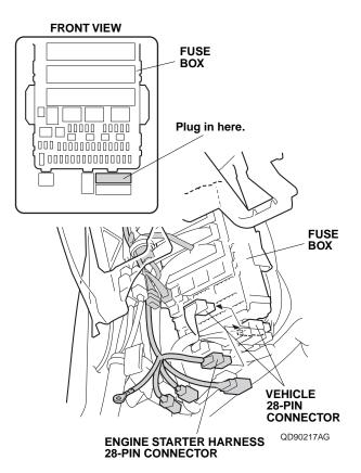
59. Release the vehicle 2-pin connectors, and install it to the vehicle connectors as shown.
