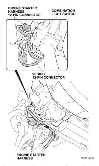
83. Plug the remaining engine starter harness 12-pin connector into the combination light switch.
