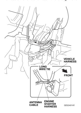
96. Bundle up the excess antenna cable, and secure it to the dashboard with the one wire tie loosely installed in step 87.
