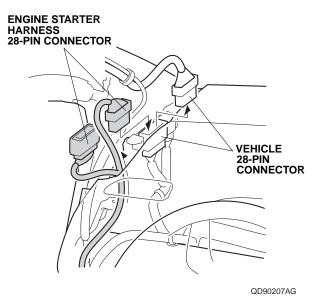
43. Route the engine starter harness 28-pin connectors as shown, and plug the engine starter harness 28-pin connector into the vehicle 28-pin connector.
