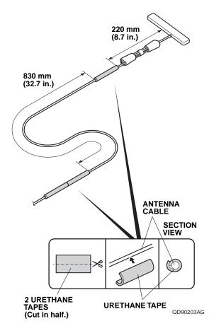
27. Wrap two halves of urethane tape around the antenna cable as shown.
