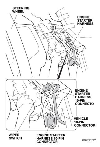
80. Plug the remaining engine starter harness 10-pin connector into the wiper switch.
