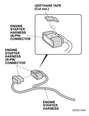
62. Plug the engine starter harness 28-pin connector to the engine starter harness 28-pin connector.
