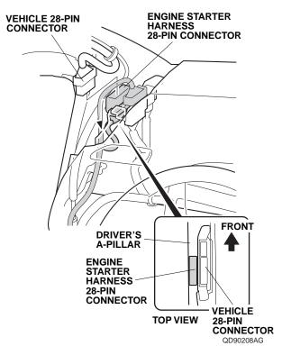
45. Plug the vehicle 28-pin connector into the engine starter harness 28-pin connector.
