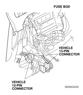
68. Remove the vehicle ground bolt.
