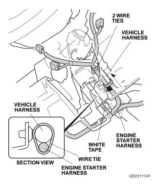
78. Align the white tape on the engine starter harness with the vehicle clip, and secure the engine starter harness to the vehicle harness with two wire ties as shown.
