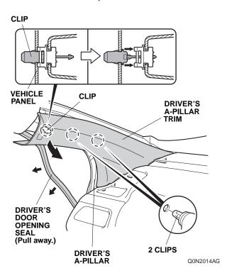
8. To prevent the clips from falling into the vehicle body, roll up the shop towel, and insert it between the driver's A-pillar and the dashboard. Take care not to damage the driver's A-pillar.
