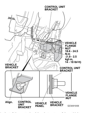
94. Install the control unit bracket on top of the vehicle bracket and align the control unit bracket with the edge of the vehicle bracket. Reinstall the vehicle flange nut. Torque the vehicle flange nut to 18.6 - 24.5 N·m (14 - 18 lbf·ft).
