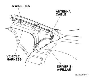
35. Secure the antenna cable to the vehicle harness with five wire ties.
