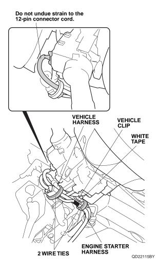
85. Route the antenna cable along the engine starter harness as shown.
