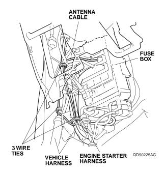
74. Route the engine starter harness under the dashboard and toward the steering wheel.
