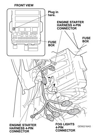
57. Plug the remaining engine starter harness 4-pin connector into the fuse box.
