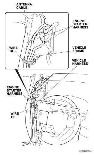
47. Secure the engine starter harness to the vehicle harness with one wire tie.
