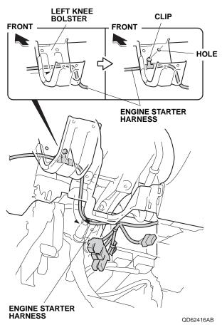
75. Secure the engine starter harness to the hole in the left knee bolster using the clip on the engine starter harness as shown.
