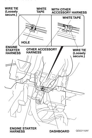
77. Route the engine starter harness along the vehicle harness as shown.
