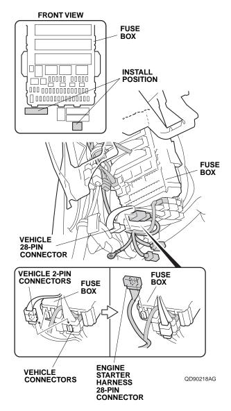
60. Slide the clip from the engine starter harness 28-pin connector onto the bottom of the fuse box, then plug the remaining vehicle 28-pin connector into the engine starter harness 28-pin connector.
